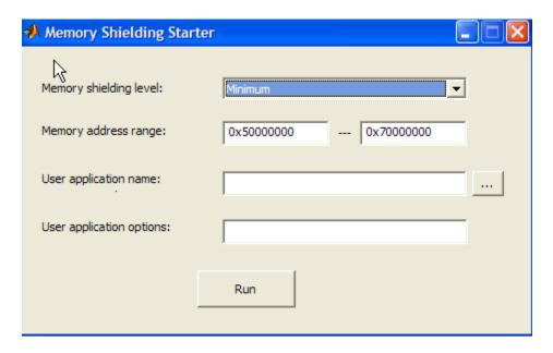
**2** Enter the appropriate values as described in MemShieldStarter Options on page 5-45. Use the default **Memory shielding level** minimum.
